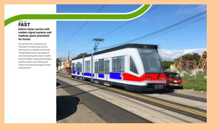
A few excerpts from the SEPTA Trolley Modernization Program Goals presentation show the above concept double-end vehicle similar to the Siemens S70/S700 vehicle now used in San Diego and other cities. It also seems to show plans to extend the pavement at trolley stops to reach the tracks, eliminating about 90 ft or 4 cars of parking spaces as shown in the next illustration.
